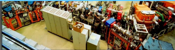
A photograph of the ion storage ring TSR at the Max-Planck Institute for Nuclear Physics in Heidelberg. It is proposed to install this ring at the HIE-ISOLDE facility in CERN, thus enabling a variety of unique experiments in nuclear-, astro- and atomic physics.
