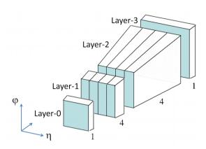
Each trigger tower segmented into 10 supercells, with 4 depth layers and 4  $\eta$  strips in middle two
