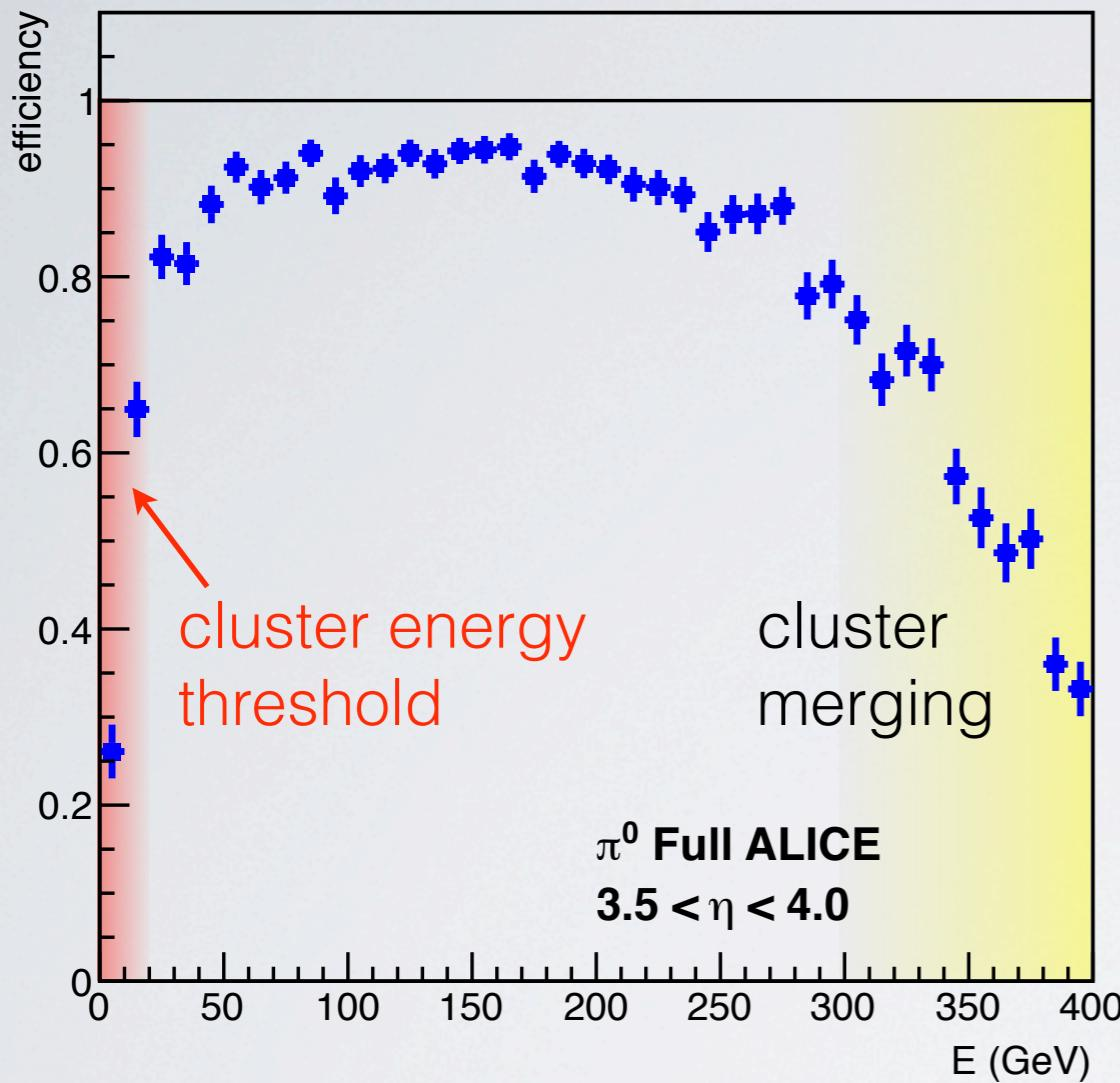
single particle simulation in full ALICE setup, good efficiency up to  $E \approx 300$  GeV ( $p_T \approx 10$  GeV/c)
