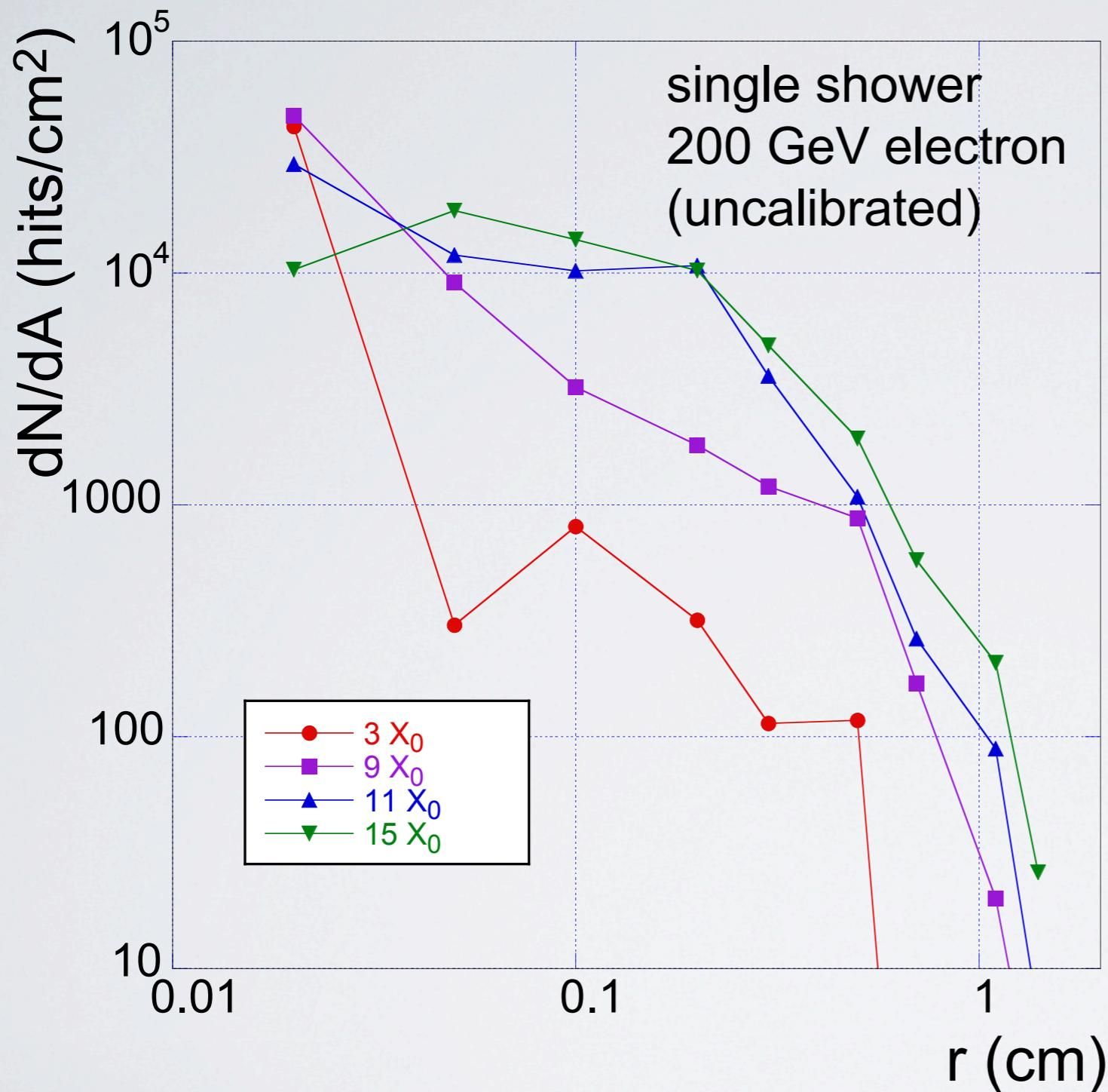
high granularity allows detailed measurements of shower distribution below the mm scale
