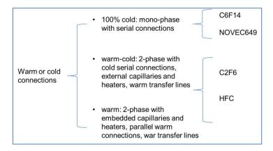
In simple terms, we should decide whether or not the end-cap zone has enough space for insulated module (inter-)connections. Then we choose an appropriate simple and "as COTS as possible" cooling technology (probably, sacrificing costs over robustness and performance) and focus the design efforts on the optimal module-end structure for this cooling method. Eco-friendliness is a desirable but not fundamental factor in this logic.
