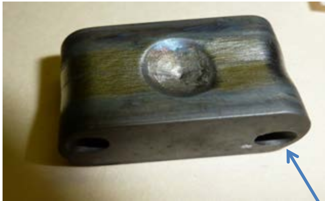
Mo-Cathode: Thermocouple location
