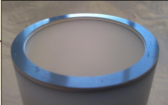
New Ceramic with braze metal ring
