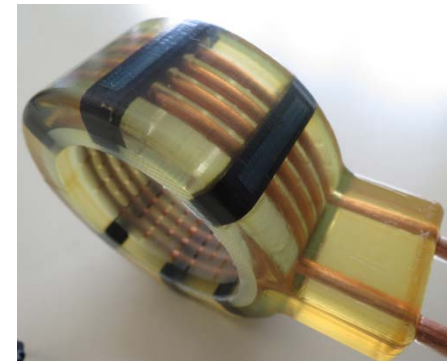
3D-printing of the solenoid Epoxy mould
