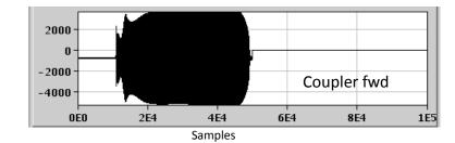
Forward & reflected signals are demodulated in software into I (in-phase) and Q (quadrature):
