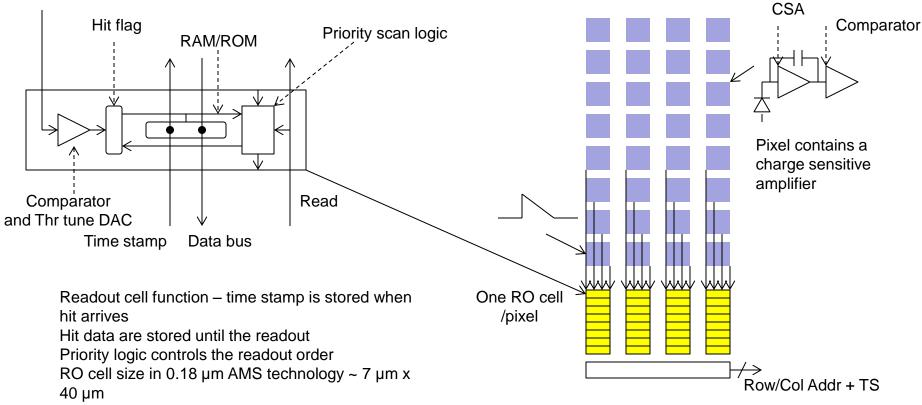
(with comparator and threshold-tune DAC)
