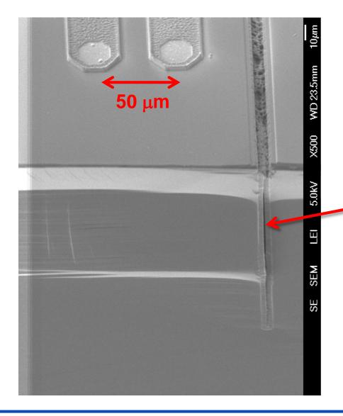
During polysilicon deposition, the trench gets filled and sealed close to the surface, leaving a narrow unfilled gap deeper into the bulk. This allows separating the devices along the trench after the substrate is thinned.
