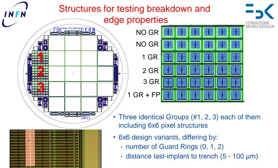
On each structure, an array of 30 × 4 pixels, shorted together by metal lines, to facilitate testing
