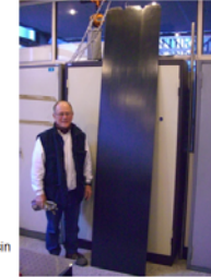
long layer of 3 alveoli demolded nov 12th with new system woven-resin (C202+ET445)
