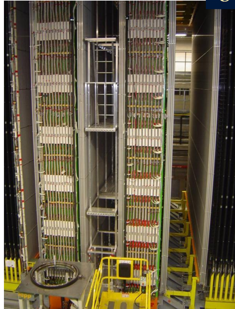
3050 m 2 Resistive Plate Counters 2000 tons of iron for the two magnets
