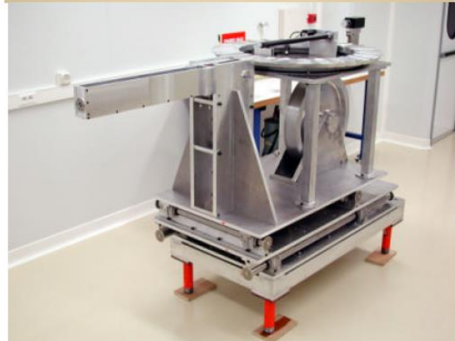
"Carousel" brick dispensing and storage system
