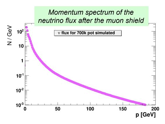
2×10⁴ neutrino interactions per 2×10²⁰ pot in the decay volume at atmospheric pressure → becomes negligible at 0.01 mbar
