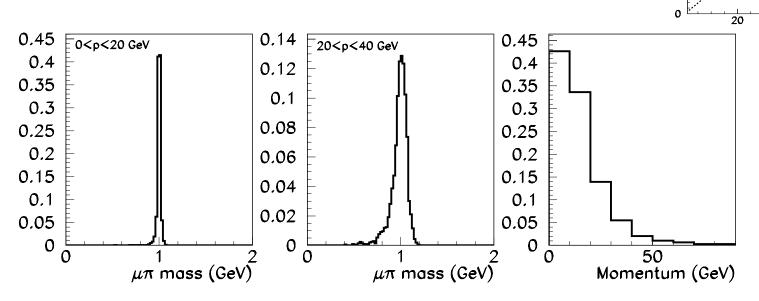
• For 0.5 Tm field integral  $\sigma_{mass}$  ~ 40 MeV for P < 20 GeV
