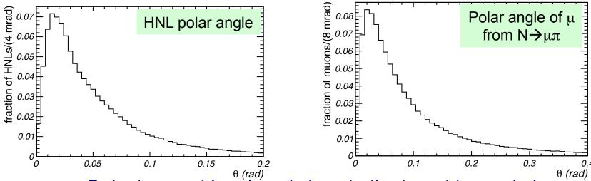
Detector must be placed close to the target to maximize geometrical acceptance
