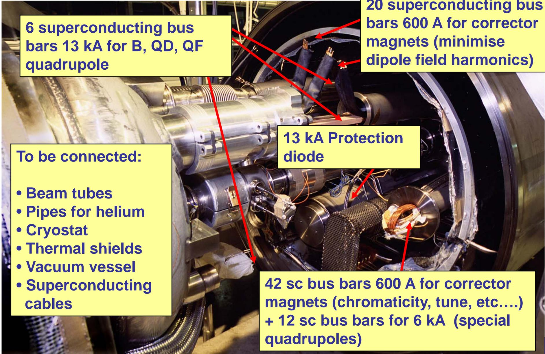
6 superconducting bus bars 13 kA for B, QD, QF quadrupole
