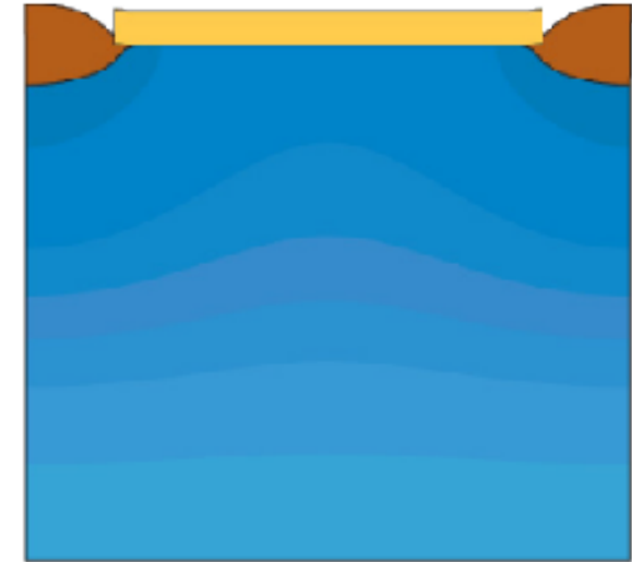
B. Anneal and field oxide growth
