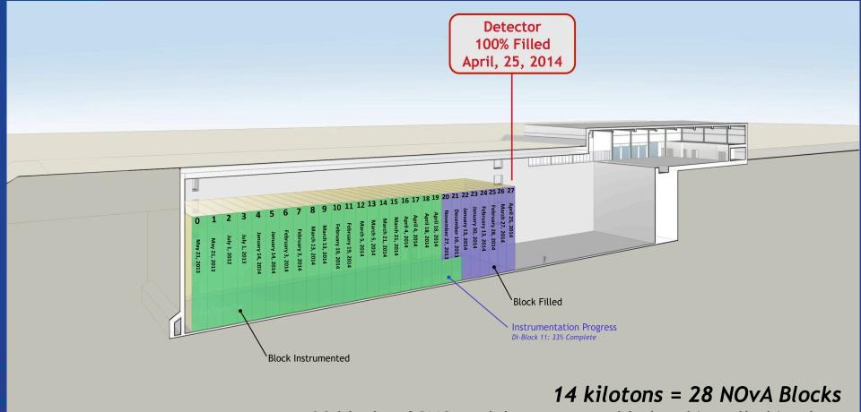
28 blocks of PVC modules are assembled and installed in place 28.0 blocks are filled with liquid scintillator 20.66 blocks are outfitted with electronics
