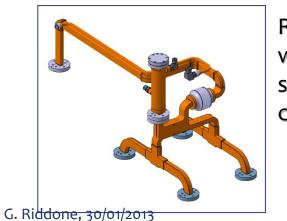
RF network: waveguides and several RF components
