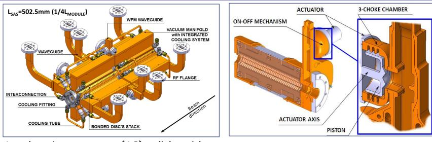
Accelerating structure (AS) – disks with 4 manifolds and all needed technical systems
