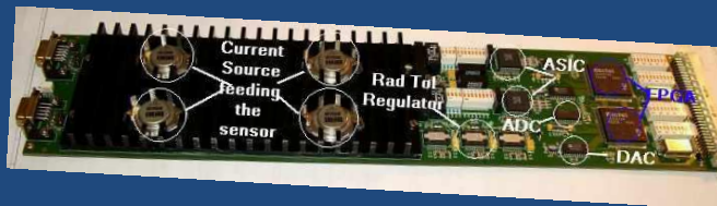
RadTol in-house electronics for signal conditioning and actuation
