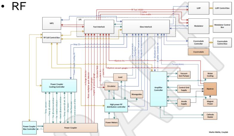
Figure 1: RF Cell Control & Protection systems
