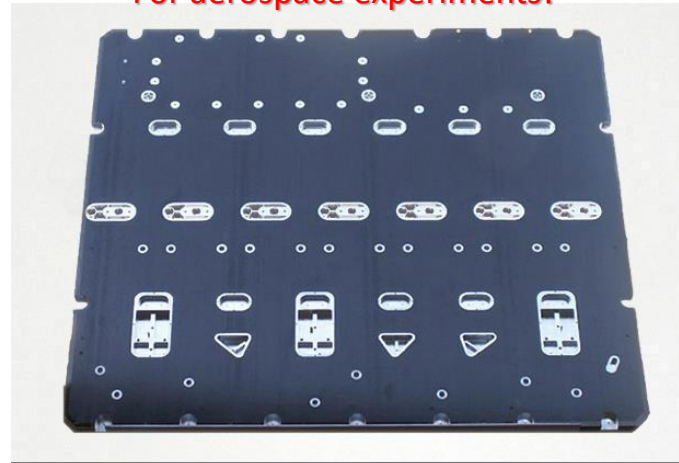
L-BAND SAR Sandwich pannel (1100 X 1000) CFRP — Alu. honeycomb — CFRP
