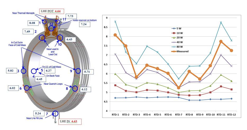
Measured cold mass surface temperatures correspond to a model uniform heat load between 40 and 80 W. Measured heat load was ~75W
