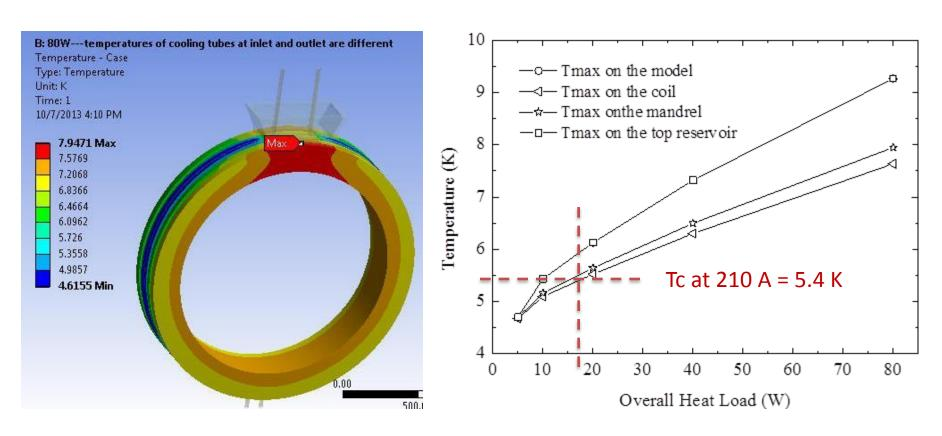
Heat Load needs to be < 15 W for coil Tmax < 5.4 T (the critical temperature at 210 A)
