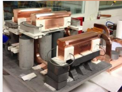
Mo spring to hold manifold & cover
