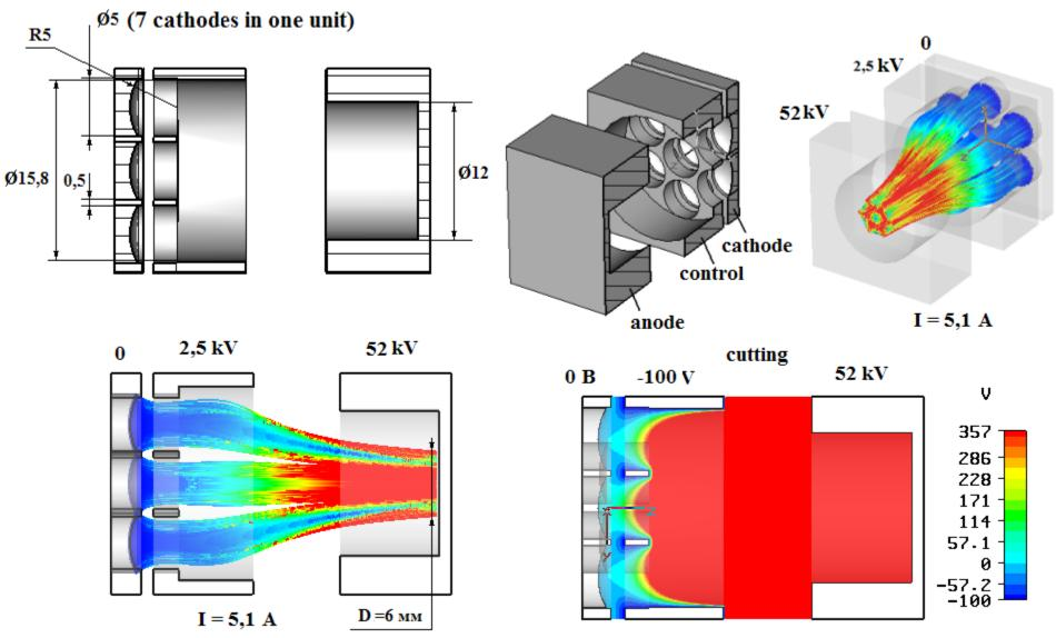
Cut voltage for central channel U= -220 B
