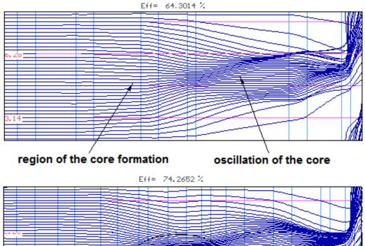
Traditional bunching – six cavities, oscillation of the core is in the long drift tube between fourth and fifth gaps.
