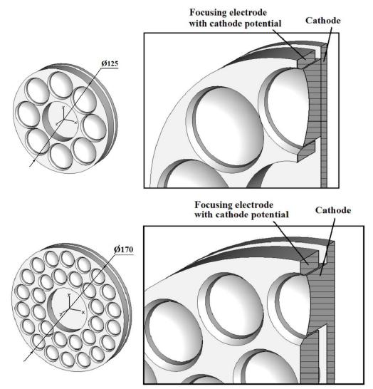
Variant 1 Number of beams 8, Pulsed current 155 A, Cathode diameter 35 mm, Cathode loading, 2,0 A/cm<sup>2</sup>
