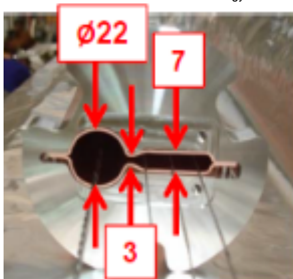
NEG coating of exotic vacuum chambers, for MAXIV
