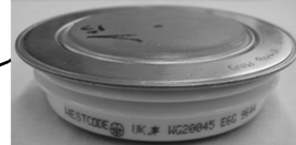
GTO die damaged during testing at high di/dt
