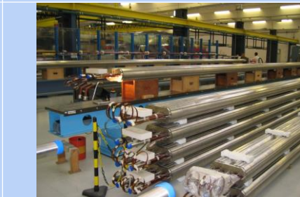
Collared coils ready for cold mass assembly
