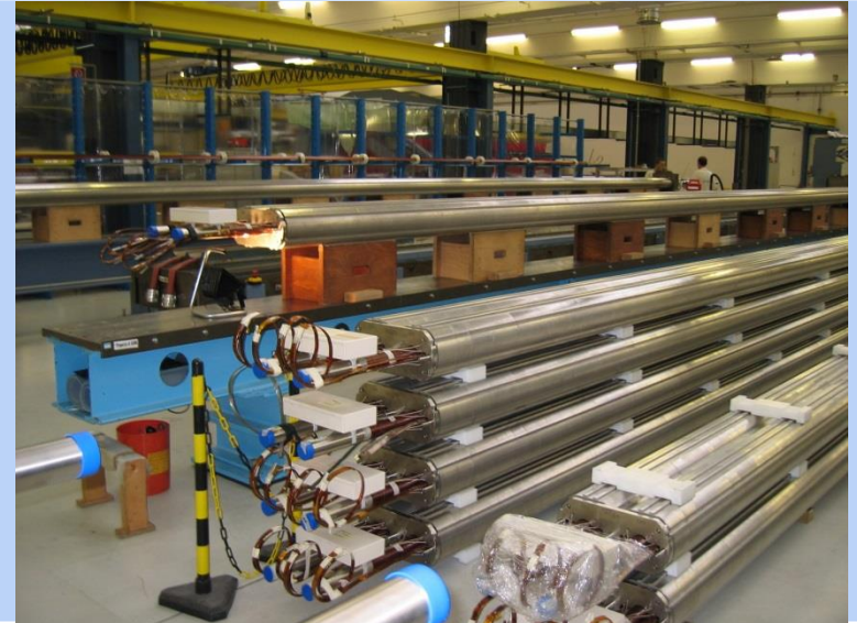
Collared coils ready for cold mass assembly
