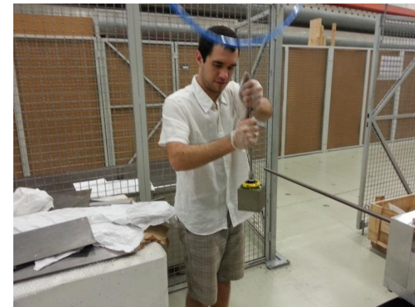
Pictured: Permanent magnet block manipulation with suction cup
