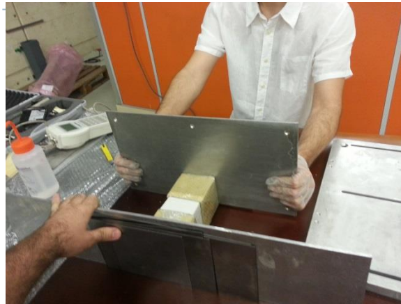
Pictured: Separation of permanent magnet blocks
