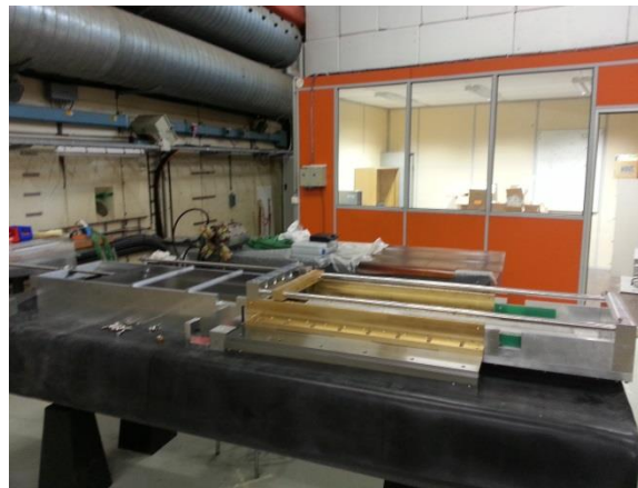
Pictured: insertion of the permanent magnet block in the magnet yoke
