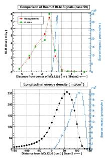
BLM dose simulation based on the original loss distribution (source) for  $8.2 \times 10^8$  protons
