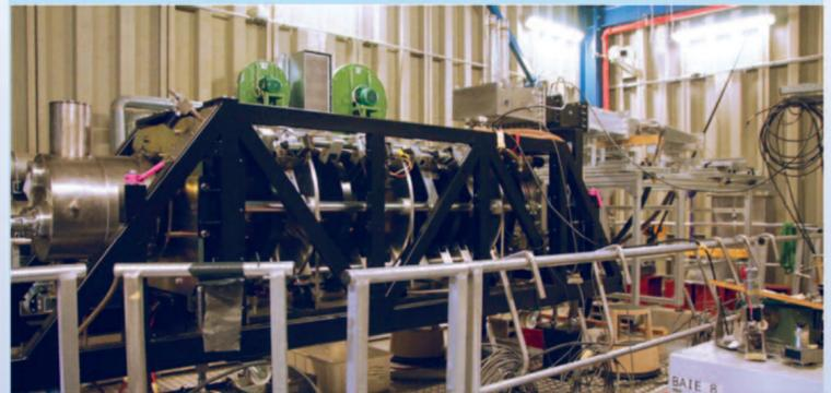
TH2182 Klystron at 704 MHz operated in SPL configuration
