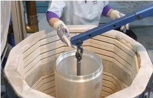
Figure 7. Blocking Capacitor/Line Assembly in Kiln
