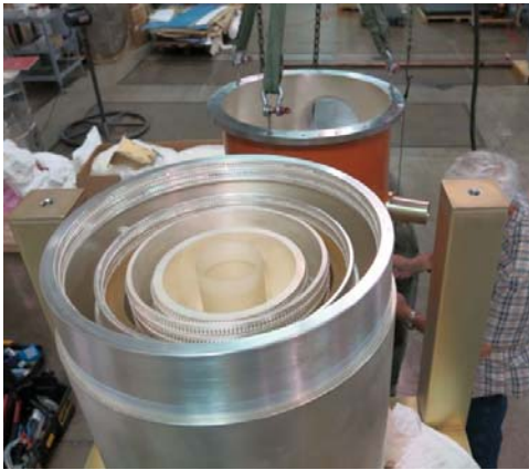
Figure 2. Nested Assemblies for Filament, g1 and g2
