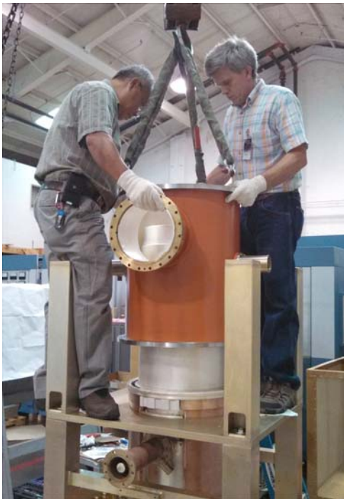
Figure 3. Installing Output Cavity
