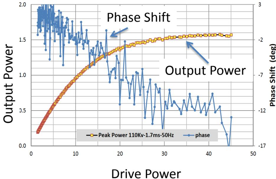
Curve 4 TH2182 001 bandwidth at P<sub>sat</sub> - 1,5dB @50Hz 1.7ms
