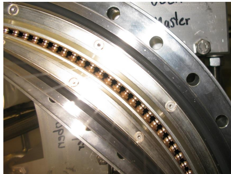
Gold plated tuner after power tests
