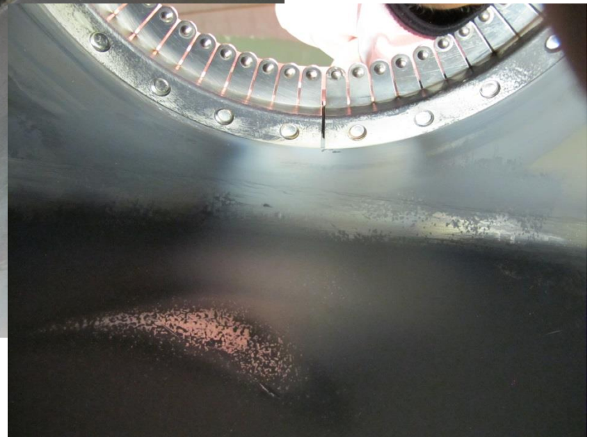
Again spot on cavity wall close to coupling loop
