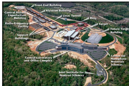
USA 2006: SNS (<1.4 MW) 1 GeV, 26 mA in linac, 627 ns long pulse, 60 Hz
