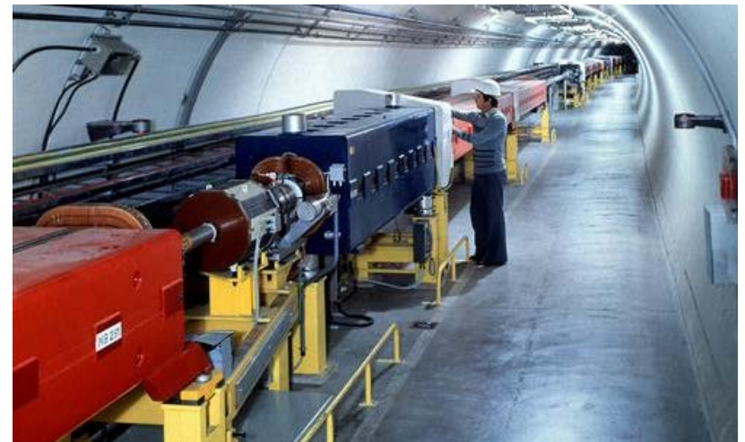
400 GeV SPS at CERN strong focussing, separated function magnets
