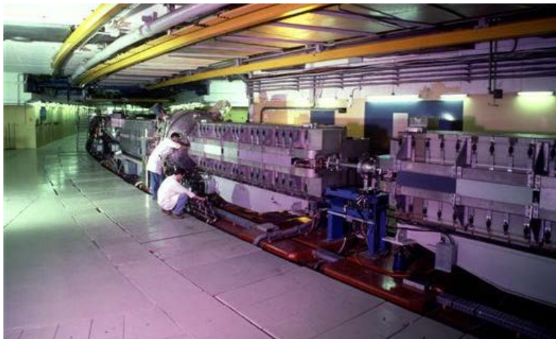
28 GeV PS at CERN strong focussing, combined function magnets
