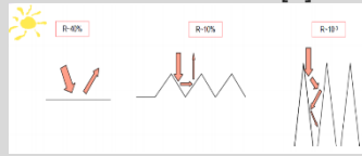
Figure 1: Reduction of reflection depending on the structure of the absorbing surface
