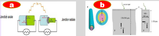
Figure 2: Representation of the axial and radial junction in a nanowire
