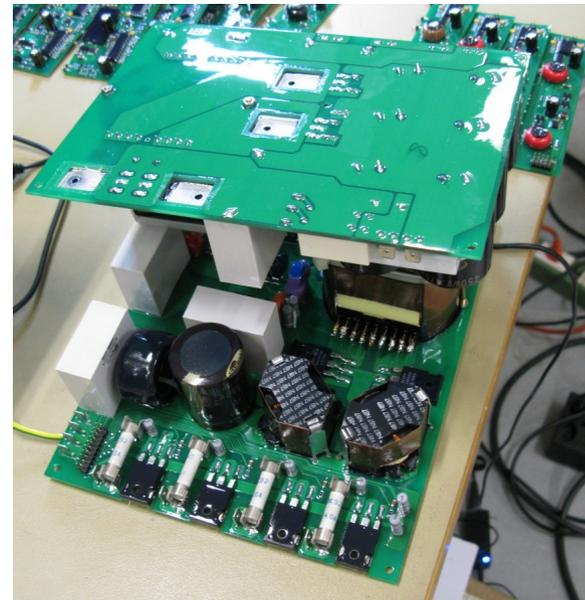
*Disassembling of HV crates, and covering with lacquer*
