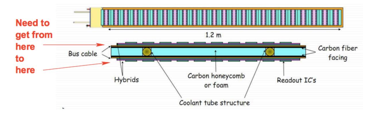
Add wrap around cable with a high-speed serial interconnect for each 128 channels
