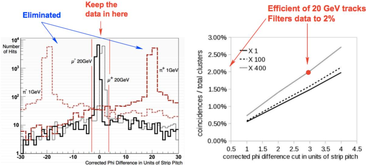
•Two-trigger layers at 0.8 m and 1.0 m have roughly double the readout rate as an offline only design
