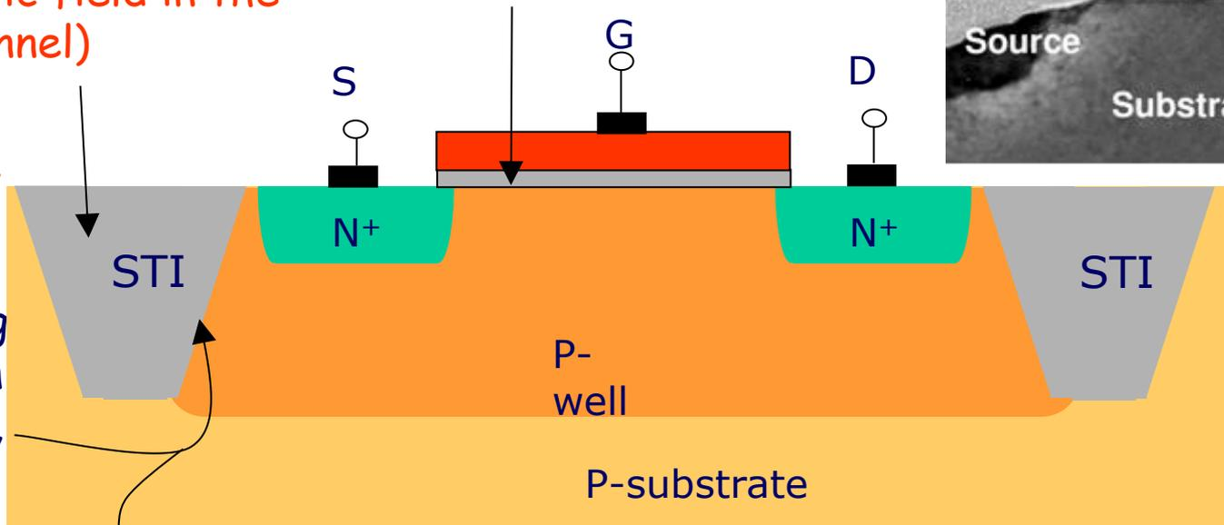
Increasing sidewall doping makes a device less sensitive to radiation (more difficult to form parasitic leakage paths)
