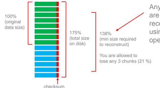
Any 11 of the 14 chunks are enough to reconstruct the data using only XOR operations (very fast)
