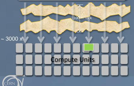
Every Readout Unit has a piece of the collision data All pieces must be brought together into a single compute unit The Compute Unit runs the software filtering (High Level Trigger – HLT)
