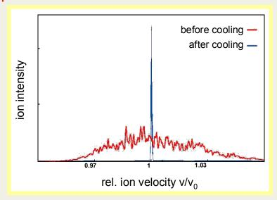
p̄-beams can be cooled → Excellent resonance resolution
