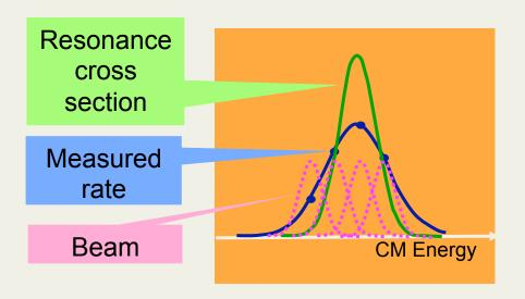
The production rate of a certain final state v is a convolution of the BW cross section and the beam energy distribution function  $f(E, \Delta E)$ :
