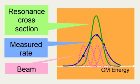
The production rate of a certain final state v is a convolution of the BW cross section and the beam energy distribution function  $f(E, \Delta E)$ :
