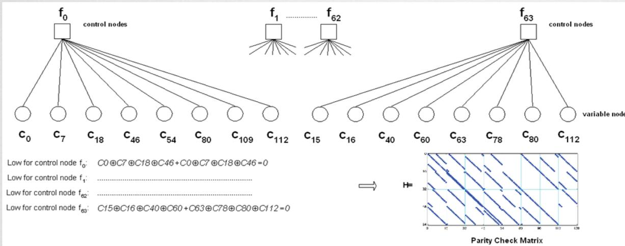
Check nodes for (128, 64) code comprises 64 check nodes, each accepting systematically 8 bit from the variable node sequence
