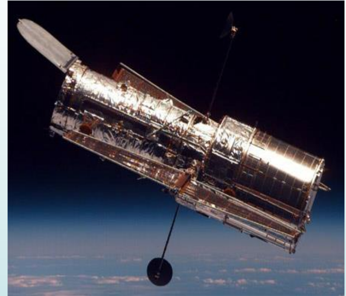
The Hubble Space Telescope (HST) is a 2.4-m (7.9-ft) aperture space telescope. It was carried into low Earth orbit by a Space Shuttle in 1990, and it remains in operation.
