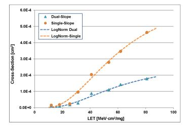
Cross-sections calculated counting as errors all the output values with deviation larger than  $4\sigma$ .
