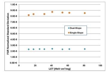
After post-processing and exclusion of the values outside  $4\sigma$ , the standard deviation is not affected by SEEs, even with the high ion flux used in the experiments (10<sup>4</sup> ions·cm<sup>-2</sup>·s<sup>-1</sup>)
