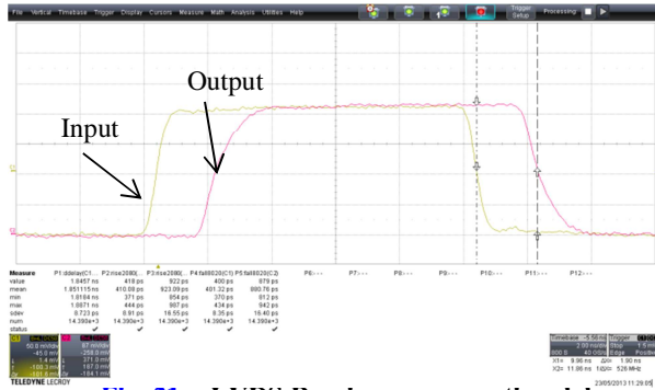
Fig. 21a: LVDS Receiver, propagation delay
