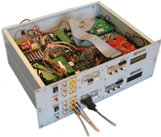
Figure 1: FPGA based MPPB hardware (credits: RECORE)
