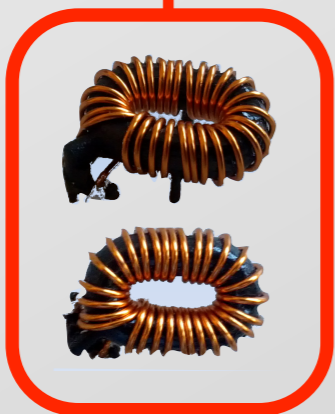
Custom air-core toroid inductor, 400nH
