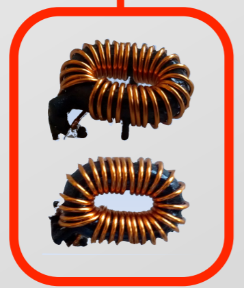
Custom air-core toroid inductor, 400nH
