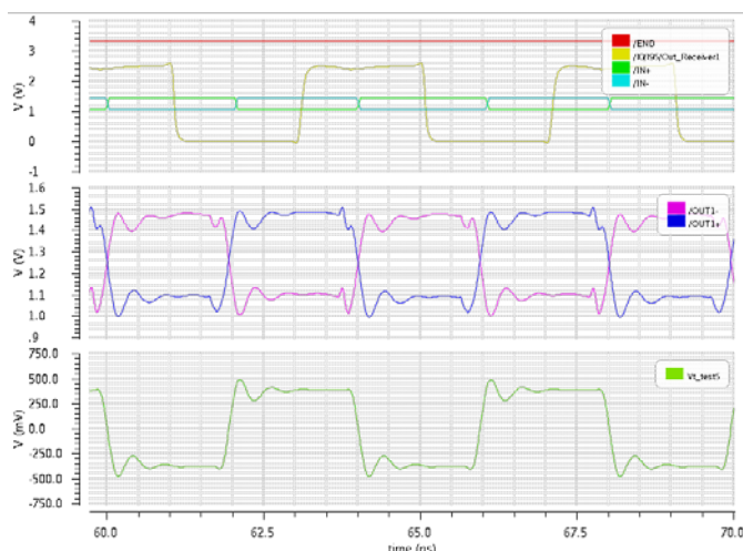
Figure 4. Driver output at nominal conditions.
