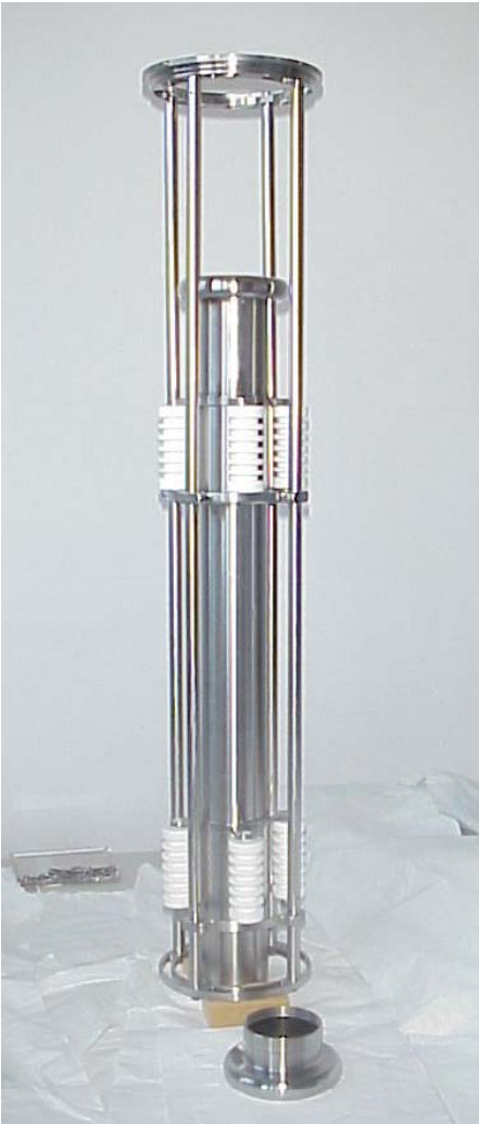
Pulsed drift tube (h = 70 cm)
